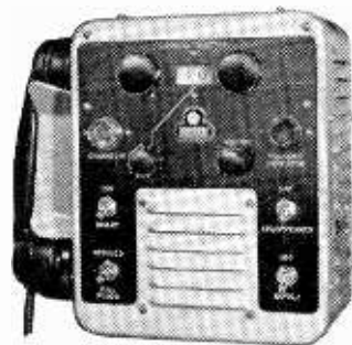
Compact control unit of the Marconi "Argonaut" marine v.h.f. radio telephone.
